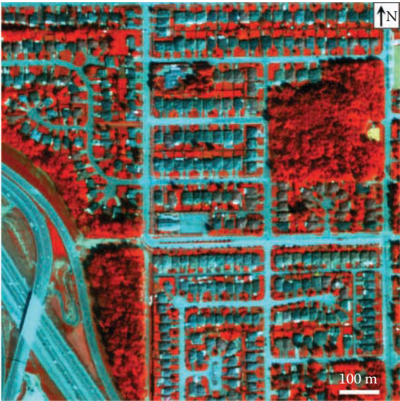
FIGURE 1.5 Color composite image created from CASI-1500 VNIR hyperspectral bands acquired in Surrey, BC, Canada, in May 2013. Band 70 (1.0273 μm) is used as red, band 15 (0.5020 μm) as green, and band 5 (0.4061 μm) as blue.
