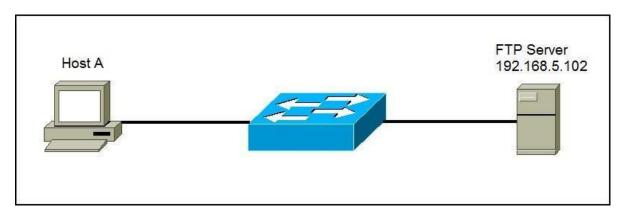
A user wants to transfer files from Host A to the FTP server. The user will start an FTP client program (in this example, FileZilla), and initiate the connection:
