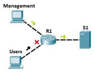
Let's say that server S1 holds some important documents that need to be available only to company's management. We could configure an access list on R1 to enable access to S1 only to users from the management network. All other traffic going to S1 will be blocked. This way, we can ensure that only authorized user can access sensitive files on S1.
