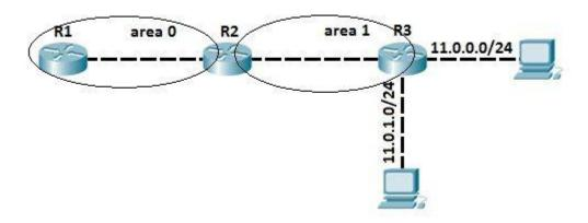
All three routers are running OSPF and exchanging routers. Before OSPF summarization is configured, the router R1 inside the backbone area has two entries for the networks 11.0.0.0/24 and 11.0.1.0/24 in its routing table.
