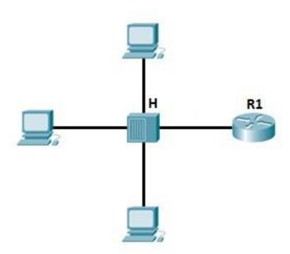
As mentioned previously, hubs create only one collision domain, so the chance for a collision to occur is high. The hub depicted above simply repeats the signal it receives out all ports, except the one from which the signal was received, so no packet filtering takes place. Imagine if you had 20 hosts connected to a hub, a packet would be sent to 19 hosts, instead of just one! This can also cause security problems, because an attacker can capture all traffic on the network.
