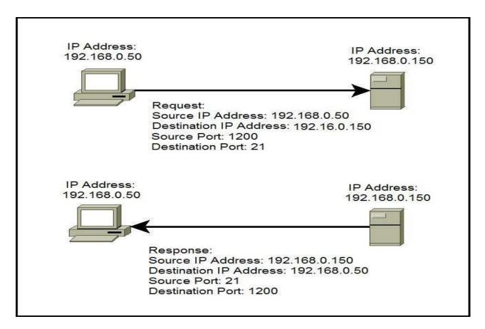
In the picture above you can see that a host with an IP address of 192.168.0.50 wants to communicate with the FTP server. Because FTP servers use, by default, the well-known port 21, the host generates the request and sends it to the FTP server's IP address and port. The host use the locally unused port of 1200 for communication. The FTP server receives the request, generates the response, and sends it to the host's IP address and port.
