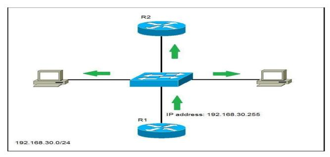
R1 wants to communicate with all hosts on the network and has sent a broadcast packet to the broadcast IP address of 192.168.30.255. All hosts in the same broadcast domain will receive and process the packet.
