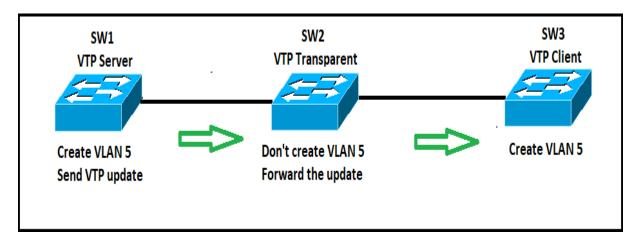
We have a simple network of three switches. SW1 is configured as VTP server. After the VLAN 5 is created on SW1, this switch will notify the connected switch (SW2) about the created VLAN. SW2 will receive the update but, since it uses the VTP transparent mode, it will not create this VLAN in its configuration. However, it will forward the VTP update to SW3. Since SW3 is configured as VTP client, it will process the update and create VLAN 5.
