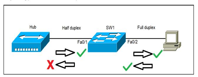
Because hubs can only operate in half duplex, the switch and hub will negotiate to use half-duplex, which means that only one device can send data at the time. The workstation on the right supports full duplex, so the link between the switch and the workstation will use full duplex, with both devices sending data simultaneously.
