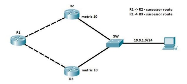
All three routers are running EIGRP. Routers R2 and R3 are connected to the subnet 10.0.1.0/24. Both routers advertise the route to reach that subnet to R1. Router R1 receives the two routing updates for the subnet 10.0.1.0/24 with the same metric (the metric is the same because both routers connect to the subnet 10.0.1.0/24 and R1 across the links with the same bandwidth and delay values). Router R1 places both routes in the routing table and load balances across three links.
