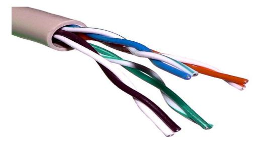
A twisted-pair cable uses 8P8C connector, sometimes wrongly referred to as RJ45 connector (Photo credit: Wikipedia).
