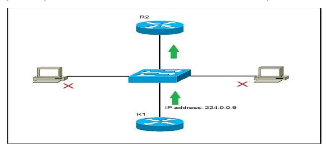
R1 has sent a multicast packet destined for 224.0.0.9. This is an RIPv2 packet, and only routers on the network should read it. R2 will receive the packet and read it. All other hosts on the LAN will discard the packet.
