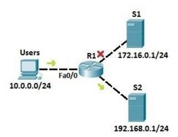
We want Users from the network 10.0.0/24 to be able to access the server S2 (IP address 192.168.0.1) and prevent them from accessing server S1 (IP address 172.16.0.1/24). First, we need to configure an access list to permit Users the access to server S2:
