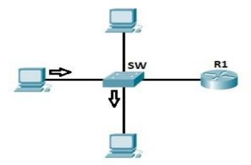
Switches increase the number of collision domains. Each port is one collision domain, which means that the chances for collisions to occur are minimal. A switch learns which device is connected to which port and forwards a frame based on the destination MAC address included in the frame. This reduces traffic on the LAN and enhances security.
