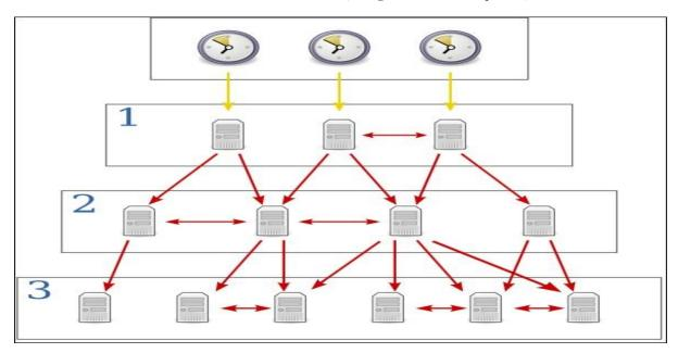
NTP uses a client-server architecture; one host is configured as the NTP server and all other hosts on the network are configured as NTP clients. Consider the following example:
