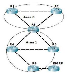
All routers are running OSPF. Routers R1 and R2 are inside the backbone area (area 0). Router R3 is an ABR, because it has interfaces in two areas, namely area 0 and area 1. Router R4 and R5 are inside area 1. Router R6 is an ASBR, because it connects OSFP network to another routing domain (an EIGRP domain in this case). If the R1's directly connected subnet fails, router R1 sends the routing update only to R2 and R3, because all routing updates all localized inside the area.
