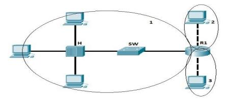
In the picture above we have three broadcast domains, since all ports on a hub or a switch are in the same broadcast domain, and all ports on a router are in a different broadcast domain.
