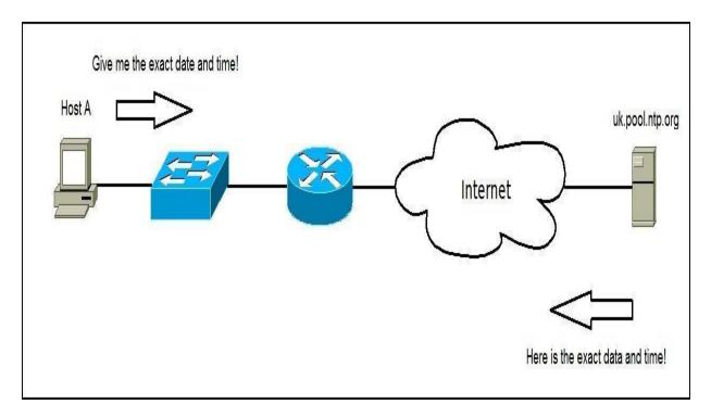
Host A is configured to use a public NTP server uk.pool.ntp.org. Host A will periodically send an NTP request to the NTP server. The NTP server will provide the accurate data and time, so Host A can synchronize its clock.
