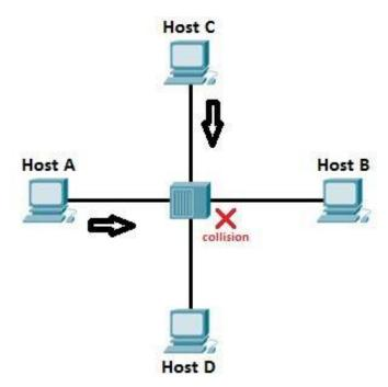
In the topology above we have a hub network. Host A is trying to communicate with host B. Host A "senses" the wire and decides to send packets. But, in the same time, host C sends its packets to host D and the collision occurs. The sending devices (host A and host C) detect the collision and resend the packet after a random period of time.
