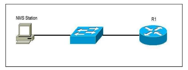
The router R1 is configured to send SNMP traps to the NMS Station. If a problem occurs, the router will send an SNMP trap to Host A. For example, if there is a port security violation on R1, the router will send the SNMP trap, notifying that there has been a potential security breach on the network.
