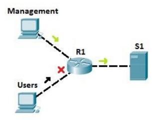
Let's say that server S1 holds some important documents that need to be available only to the company's management. We could configure an access list on R1 to enable access to S1 only to users from the management network. All other traffic going to S1 will be blocked. This way, we can ensure that only authorized user can access the sensitive files on S1.
