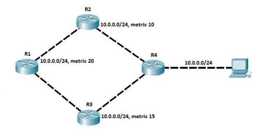
R1 has two paths to reach the subnet 10.0.0.0/24. The path through R2 has the best metric (20) and it is stored in the R1's routing table. The other route, through R3, is a feasible successor route, because the feasibility condition has been met (R3's advertised distance of 15 is less than R1's feasible distance of 20). R1 stores that route in the topology table. This route can be immediately used if the primary route fails.
