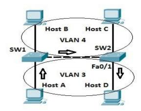
There are two VLANs in the topology pictured above, namely VLAN 3 and VLAN 4. Host A sends a broadcast packet to switch SW1. Switch SW1 receives the packet, tags the packet with the VLAN ID of 3 and sends it to SW2. SW2 receives the packet, looks up at the VLAN ID, and forwards the packet only out the port Fa0/1, since only that port is in VLAN 3. Host B and host C will not receive the packet because they are in different VLAN than host A.
