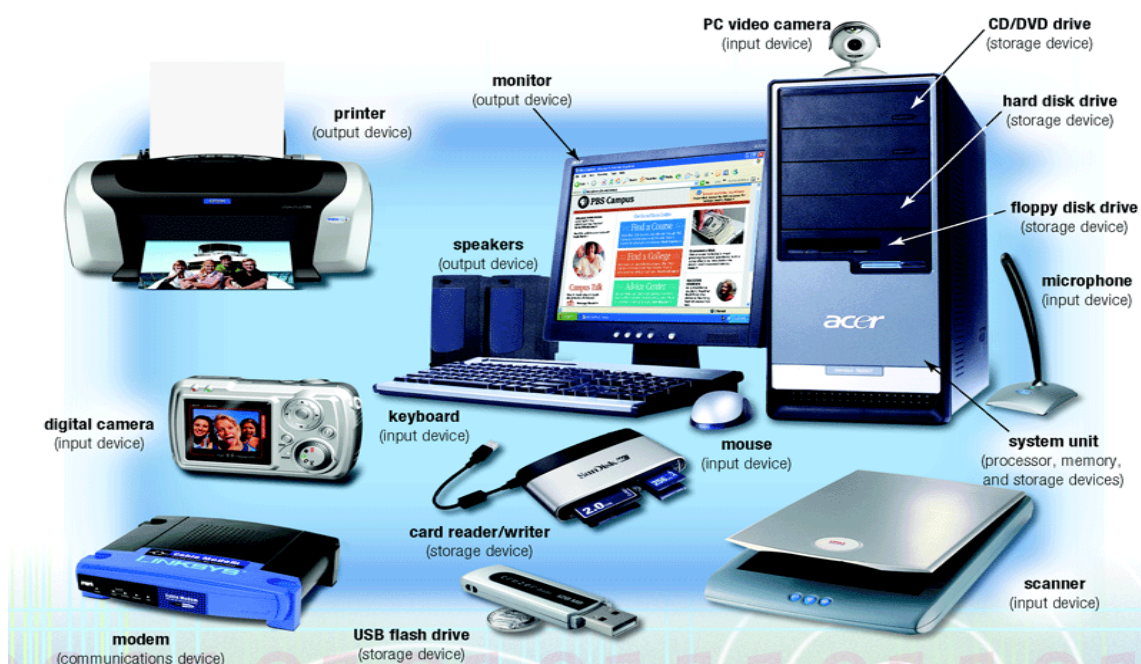
FIGURE 1 Common computer hardware components.
