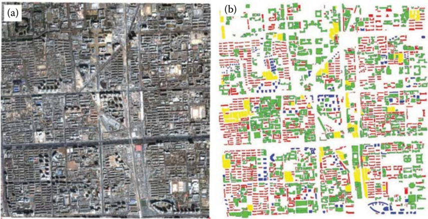
FIGURE 10.16 (a) QuickBird image and (b) the reference building objects, which are classified into four categories. (From Guo, Z., & Du, S. 2016. GIScience & Remote Sensing , 54(1), 38–63.)
