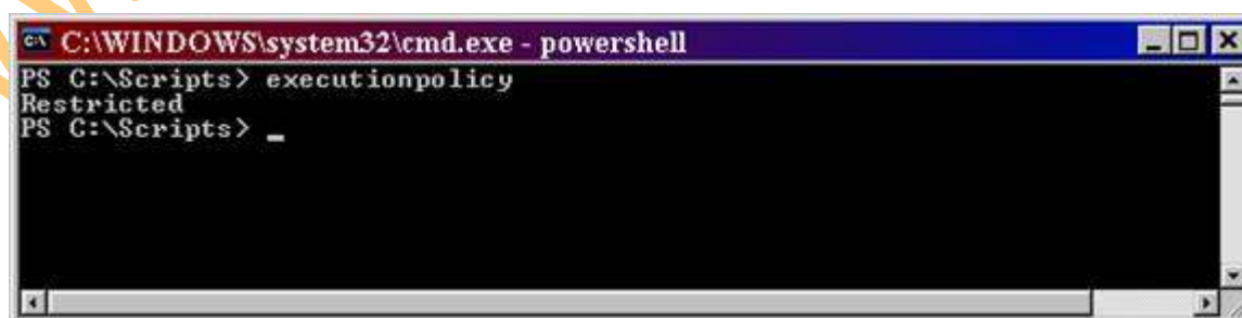
Figure 3: The Execution Policy by default is set to Restricted to secure the execution of remote PowerShell scripts
