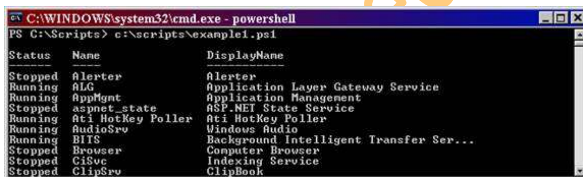
Figure 2: When the path is included with the script, the script runs without a hitch
