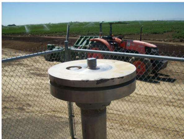
Fig. 6.4 Antenna mount without a GNSS antenna
