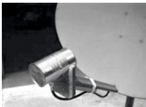
Figure 4.10: Feed horn made from a food can.
