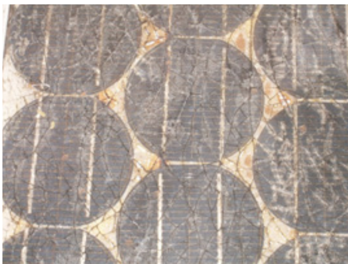
Figure 7.6: The effect of water and corrosion in a solar panel
