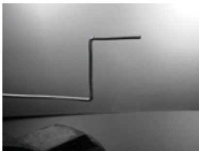
Figure 4.16: Bend the wire into a "Z" shape.
