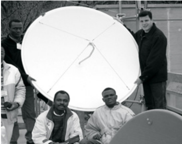
Figure 4.11: A solid dish antenna.
