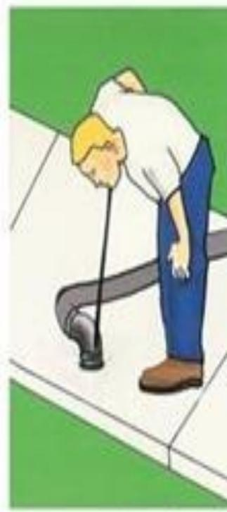
2 Slurry is pumped under the slab
