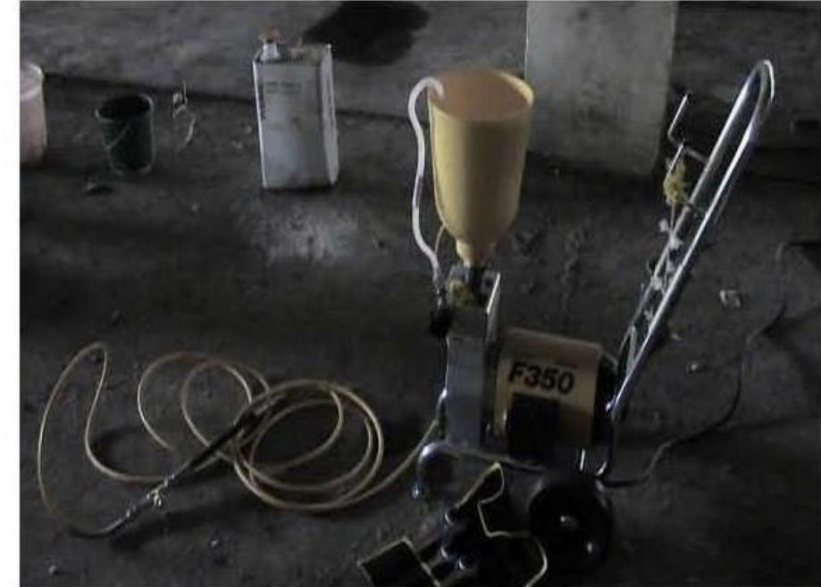
**Figure 3.** High pressure Injection Pump
