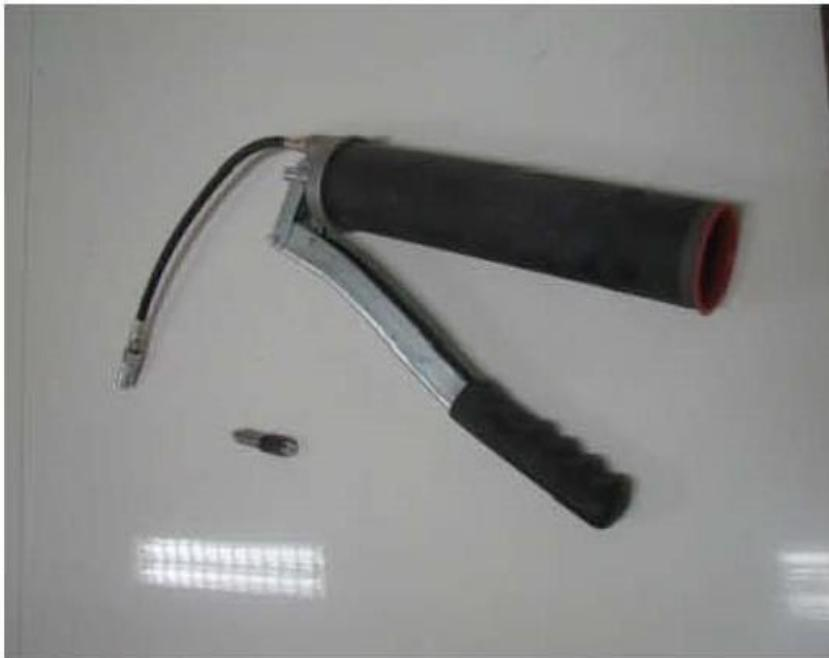
**Figure 2.** Packer and Injection Hand Pump
